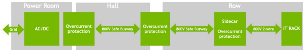
NVIDIA 800 VDC architecture minimizes energy conversions [1]
