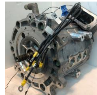
Completed ADTP IPMSM
