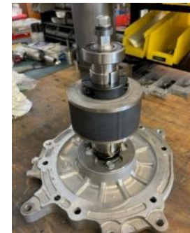
HF-10 rotor lamination stack
