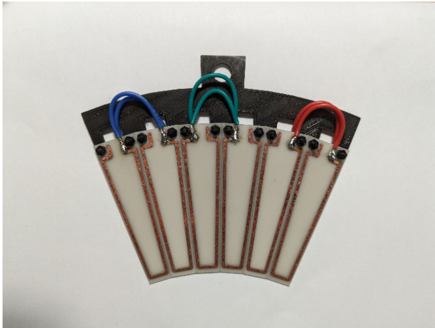
Coils of three phases forming a pole
