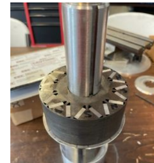
Magnet insertion with adhesive
