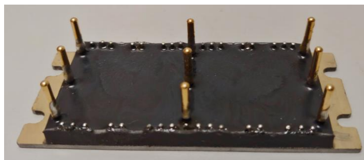
Fabricated half-bridge module.
